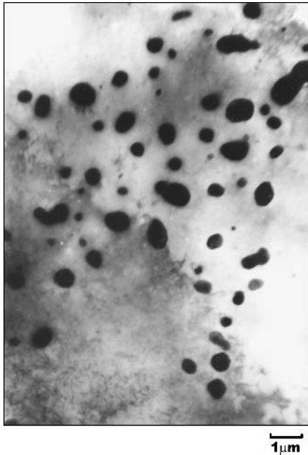
Fig. 6 TEM micrograph showing the bright field image of carbides in the sample annealed as per cycle 6. The carbides are spherical in shape and smaller in size, 6000 \times .
