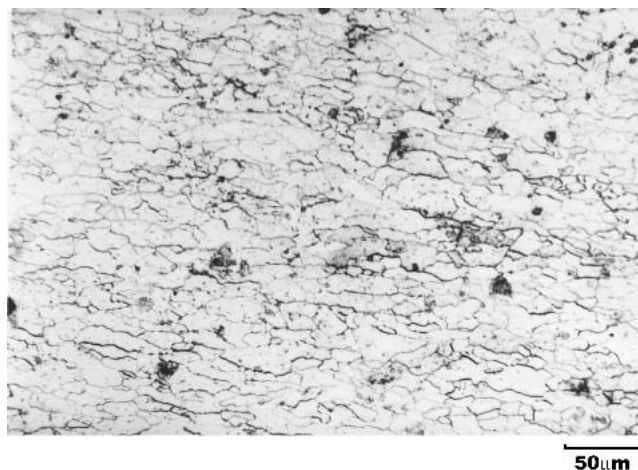
Fig. 3 Optical micrograph of the sample annealed as per cycle 3 showing mild pancaking, 200×
